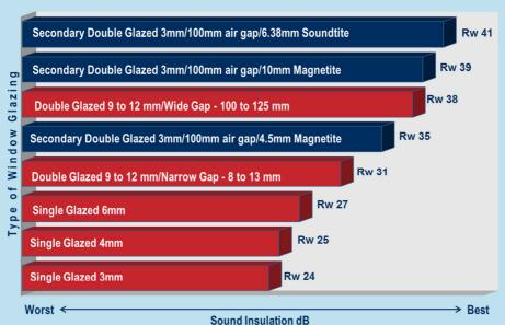
Due to a larger air cavity, secondary window systems will reduce more noise than single glazed windows and even traditional double glazed units.
